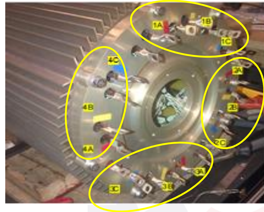
Neighbouring coils grouped into four star connected 3-phase motor units
