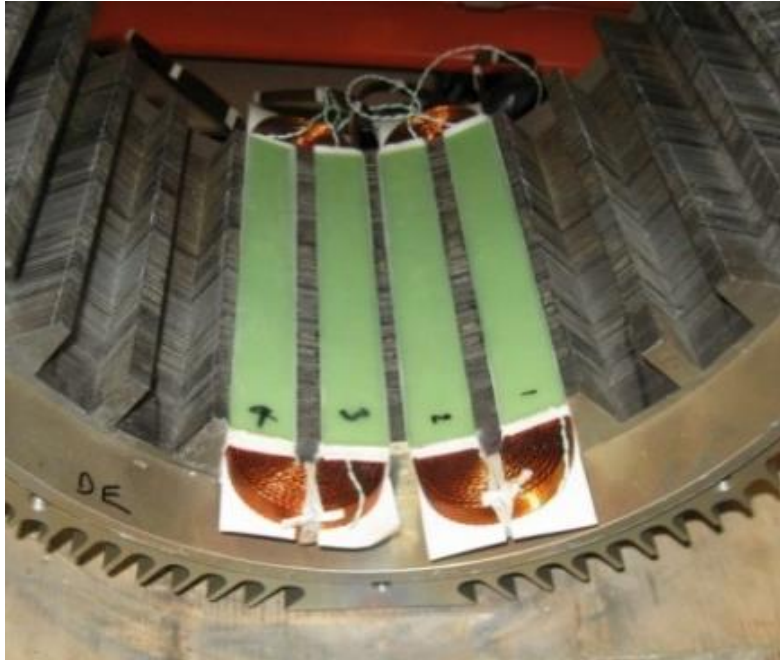
Phase coils individually terminated (and instrumented with thermocouples)
