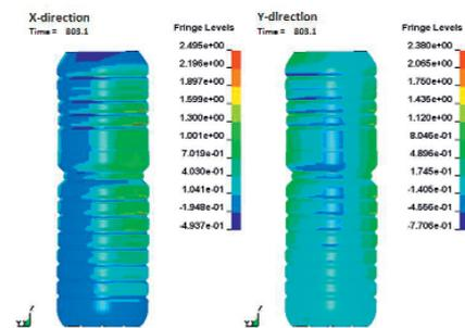
Fig. 5: Deformation of the bottle body in mm
