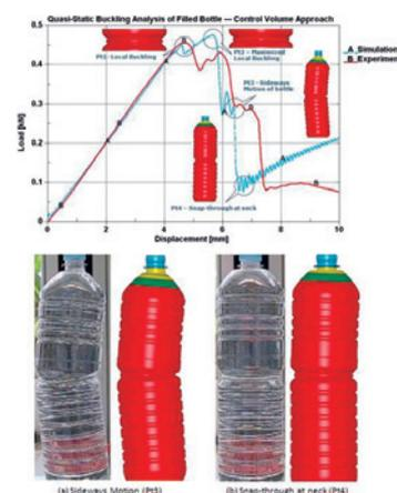
Fig. 3: Structural Response of Filled Bottle
